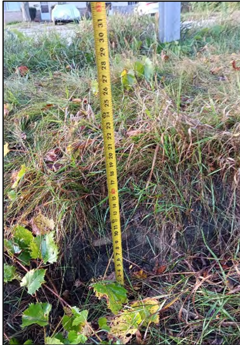
Photo 4 - Displacement of approximately 18 inches, apparent head scarp, near top of slope and guardrail
